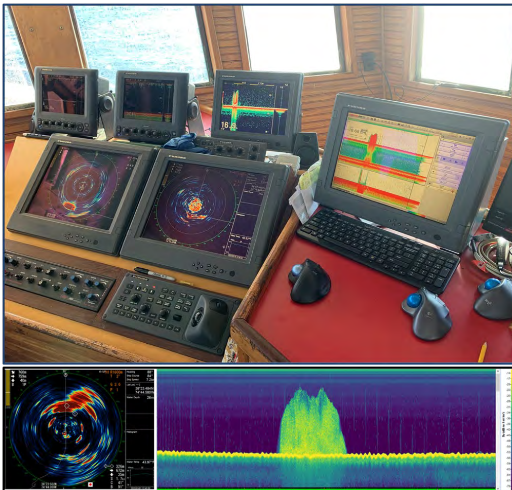
Figure 3. (Top) Instrumentation and sonar displays at helm of 49-m commercial midwater trawling vessel, F/V Dyrsten, equipped with a recordable 38 kHz Simrad ES80 split-beam echosounder and a Furuno FSV25S omnidirectional sonar. (Bottom) Paired Furuno omnidirectional (left) and ES80 echosounder (right) images of ensonified School 49.
