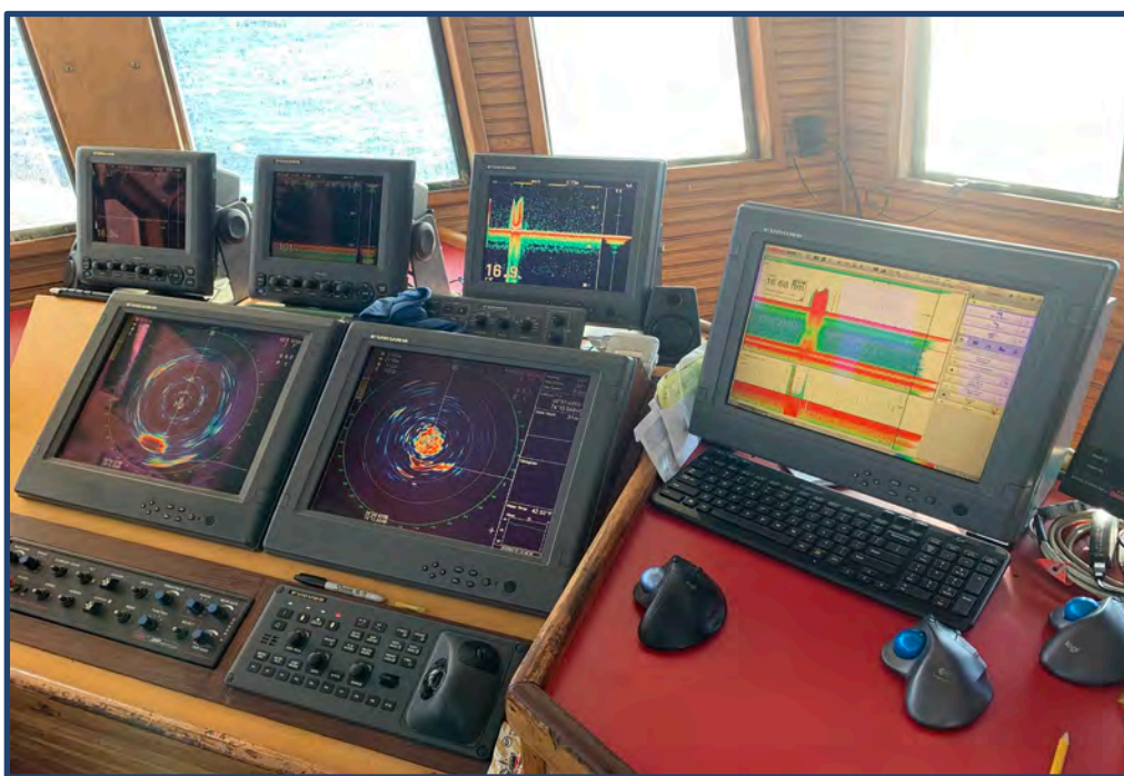
Figure 1-2 (Top) 49-m commercial midwater trawling vessel, F/V Dyrsten , equipped with a recordable 38 kHz Simrad ES80 split-beam echosounder and a Furuno FSV25S omnidirectional sonar. (Bottom) Instrumentation and sonar displays at the helm.
