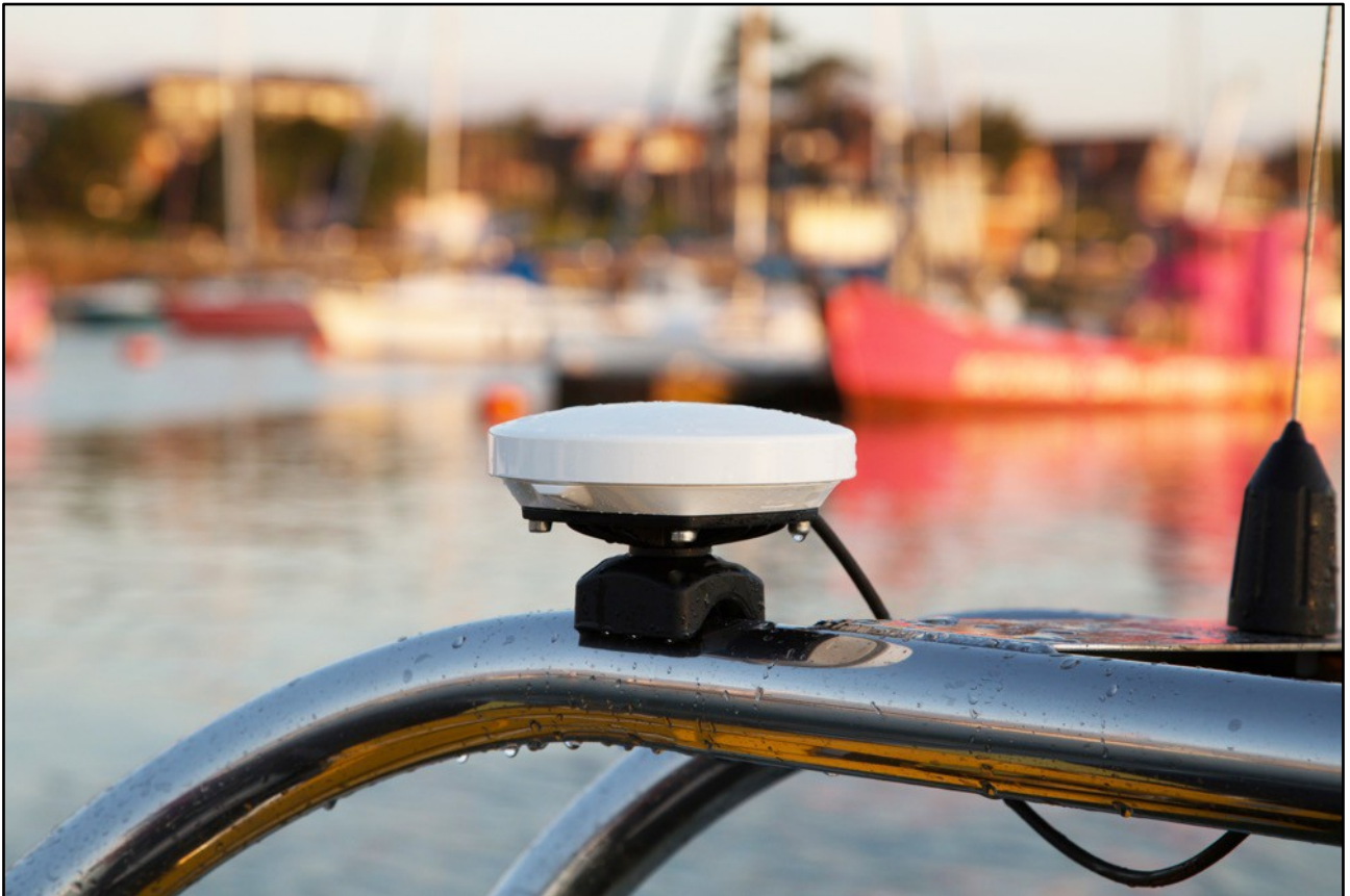
The RockFLEET unit, mounted on a tender vessel
