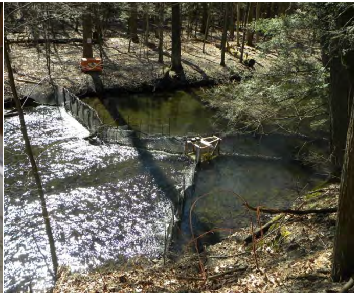
Figure 10. Top: Front view of the counter head that consists of eight four inch PVC tubes fitted with three stainless steel clamps, acting as sensors that measure water conductivity. Bottom left: View of fish counter head during construction. Bottom right: View of in-stream weir and fish counter.
