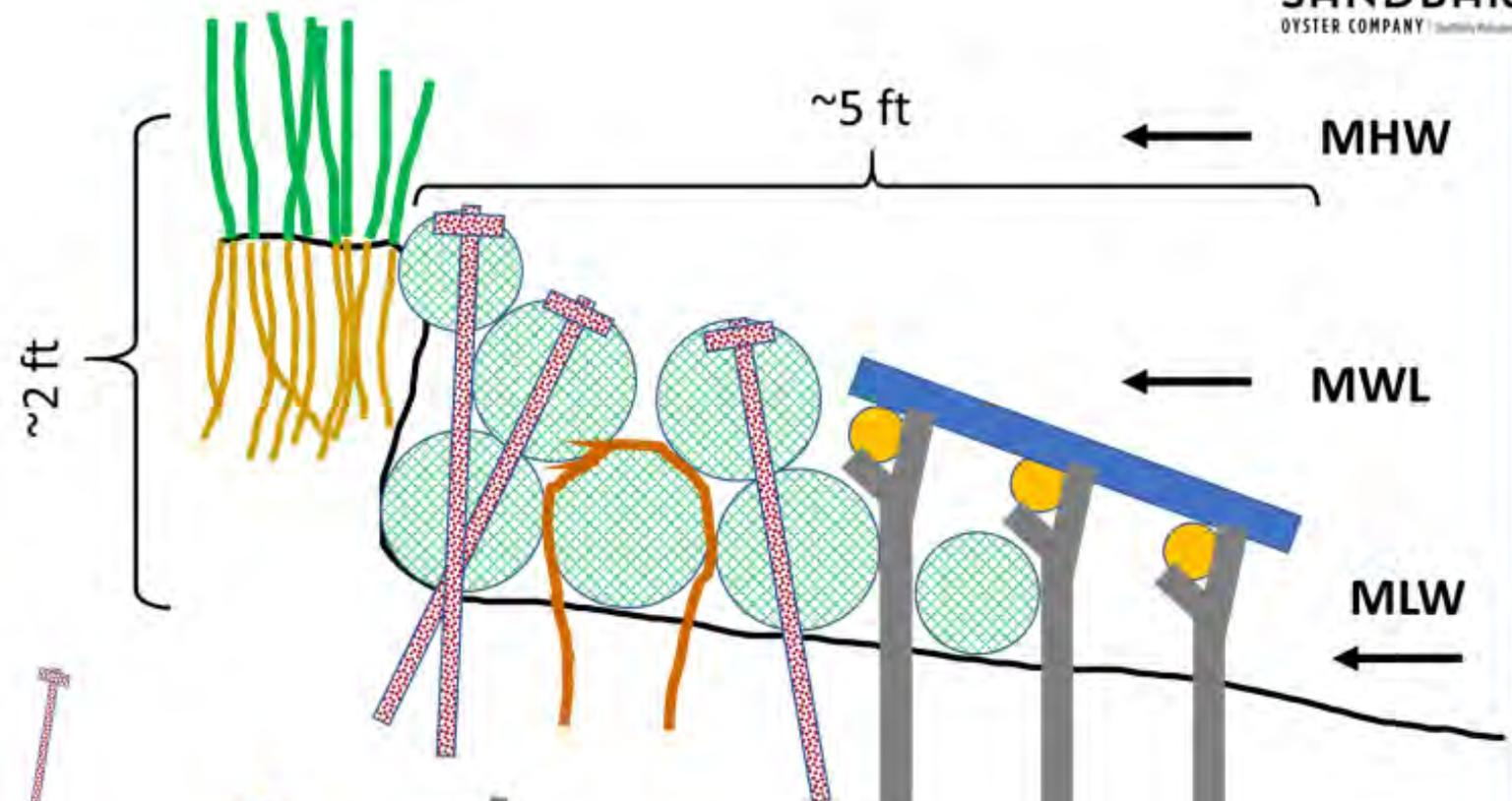
temporary rebar pin – set as shown at ~4 ft intervals; each ~3 ft long
