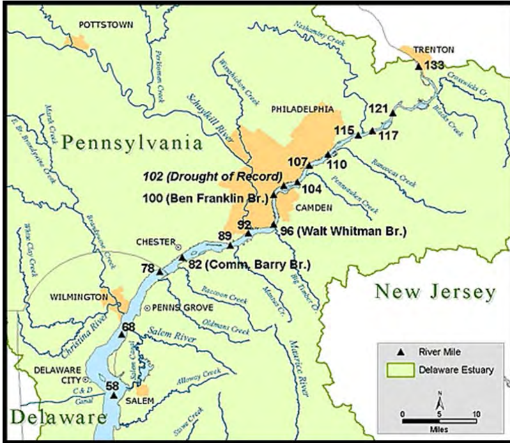
Figure 2: Historical and present day generalized location of the salt front. During the drought of record in the mid-1960's, the salt front reached river mile 102, just upriver from the Ben Franklin Bridge (rm 100). The present day location of the salt front is located at river mile 69.
