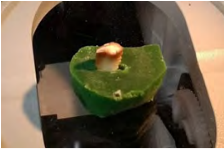
Figure 7.5 A broken and burnt otolith placed on a plasticine block to be examined under a microscope.
