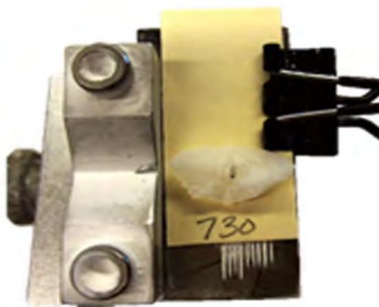
Figure 3.29 Cardstock with whole otolith attached to chuck with binder clip for sectioning using the multi-blade sectioning technique.
