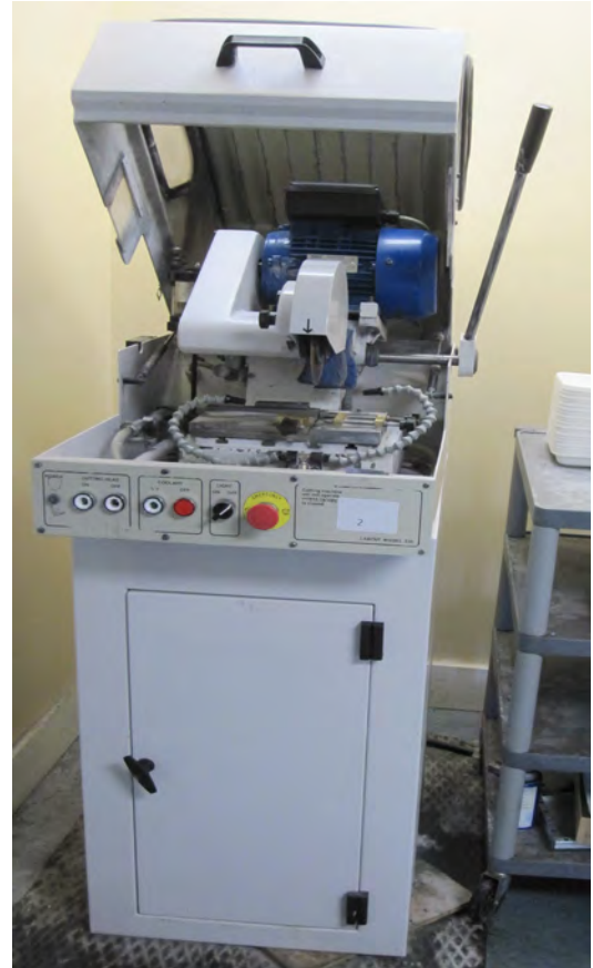
Figure 12.4.1 Benetec® L250 high-speed saw. Sectioned blocks are rinsed with water and placed in protective trays until they are labeled and secured to a large slide from which they will be aged.
