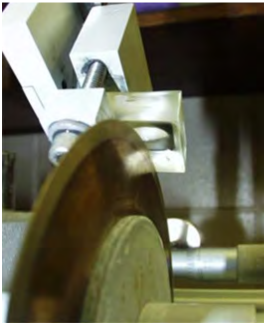
Figure 3.24 Embedded otolith mounted in low speed saw with resin block with otolith oriented against a blade at 90°.
