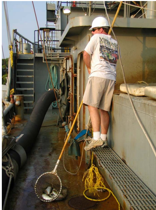
Figure 1. Port agent acquires sample (first cluster) from the top of the fish hold on a reduction purse-seine vessel using a dip net; alternately, a bucket is sometimes used.
