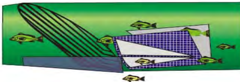
Figure II-4.2.3. Diagram of the Composite Panel BRD, which consists of two panels installed in the lower part of the extension. The panels taper inward creating a slow flow area that allows escapement of fish through two triangular escape openings cut into the extension on each side of the trawl. Each composite panel is comprised of two overlapping panels, a diamond mesh panel (interior) and a square mesh exterior panel. The inner panel reduces the water flow creating the slow flow necessary for fish escapement. The outer square mesh panel provides support, preventing the panels from billowing outward and closing off the escape openings. (NMFS)
