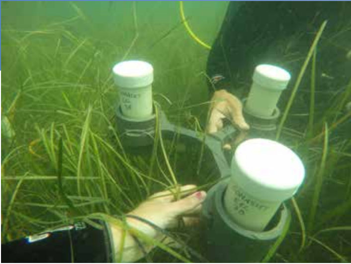
Sediment traps being deployed. Caps are removed once they are deployed. Photo credit: Dan Arsenault
