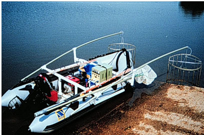
Figure 150. The electrofishing raft used to collect adult shad for shad hatchery operations and spawning stock sampling.
