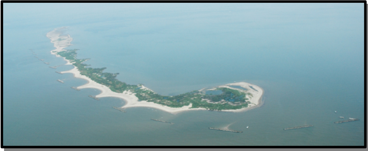
Figure 12: Segmented breakwater and scalloped (tombolo) shoreline on Raccoon Island, Louisiana (Photo credit: USDA)
